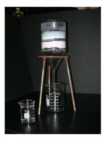
Petro Barrier column after being plugged by the addition of oil. 250 mL of water on top.
